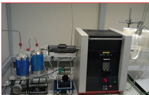
Figure 2-1 Experimental set-up scheme and image for the in-situ catalytic pyrolysis upgrading of biomass
