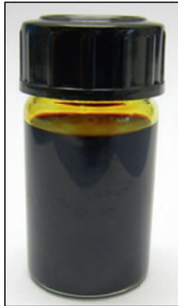
Figure 1-3 Bio-oil from pyrolysis of pinewood after extraction of aqueous phase
